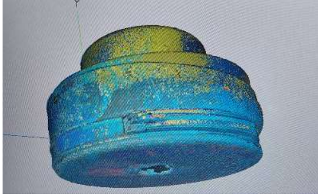
Figure 2. 3D model of PM 2 mine projection 2 Source: Authors
